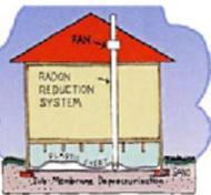
Exact system design will vary from house to house dependent upon foundation type and building materials however most will consist of PVC pipe suction points attached to a fan pulling air from under the slab foundation or membrane and disposing of it above the highest eave of the roof. This system depressurizes the house in comparison to the outside environment, reducing the levels of soil gas (and radon) being drawn into the house.
